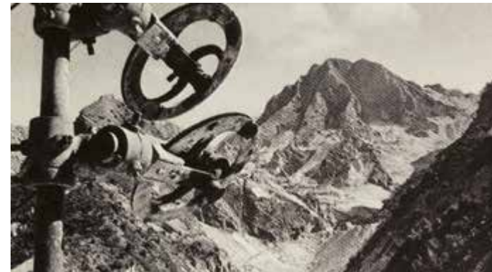
Postcard, turning pulley for saw wires in the marble quarries of Carrara.
